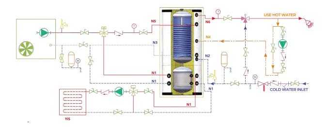
A combined water heater is a water heater that supports the production and use of heat with the possibility of using several inputs to balance the heat in the heating system, as well as the consumption of domestic hot water. The water heater saves space due to the fact that it is built into each other. Water heaters are used in houses, apartments, solar energy sources and solid fuel sources.
